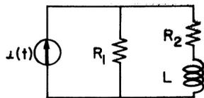
$$\frac{di_L}{dt} + \left[ \frac{R_1 + R_2}{L} \right] i_L = \frac{R_1}{L} i(t)$$
