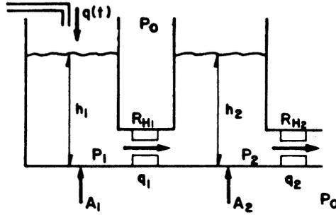
$$\frac{d^2 h_2}{dt^2} + \frac{\gamma(A_1(R_{H1} + R_{H2}) + A_2 R_{H2})}{A_1 A_2 R_{H1} R_{H2}} \frac{dh_2}{dt} + \frac{\gamma^2}{A_1 A_2 R_{H1} R_{H2}} h_2 = \frac{\gamma}{A_1 A_2 R_{H1}} q(t)$$
