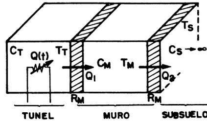
$$\frac{d^2 T_T}{dt^2} + \frac{C_M + 2C_T}{R_M C_M C_T} \frac{dT_T}{dt} + \frac{1}{R_M^2 C_M C_T} T_T = \frac{1}{C_T} Q_0(t) + \frac{2}{C_M C_T R_M} Q_0(t) + \frac{1}{R_M^2 C_M C_T} T_S$$
