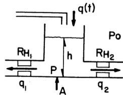
$$\frac{dh}{dt} + \frac{\gamma}{A} \left[ \frac{1}{R_{H1}} + \frac{1}{R_{H2}} \right] h = \frac{1}{A} q(t)$$
