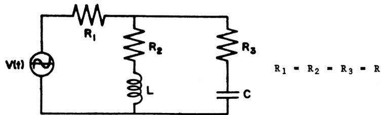
$$\frac{d^2 v_C}{dt^2} + \left[ \frac{3R}{2L} + \frac{1}{2RC} \right] \frac{dv}{dt} + \frac{1}{LC} v_C = \frac{1}{2LC} v(t) + \frac{1}{2RC} \dot{v}(t)$$
