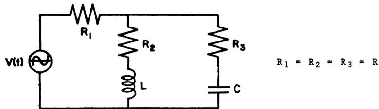
$$\frac{d^2 v_C}{dt^2} + \left[ \frac{3R}{2L} + \frac{1}{2RC} \right] \frac{dv_C}{dt} + \frac{1}{LC} v_C = \frac{1}{2LC} v(t) + \frac{1}{2RC} \dot{v}(t)$$
