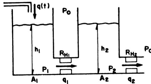
$$\frac{d^2 h_2}{dt^2} + \frac{\gamma(A_1(R_{H1} + R_{H2}) + A_2 R_{H2})}{A_1 A_2 R_{H1} R_{H2}} \frac{dh_2}{dt} + \frac{\gamma^2}{A_1 A_2 R_{H1} R_{H2}} h_2 = \frac{\gamma}{A_1 A_2 R_{H1}} q(t)$$
