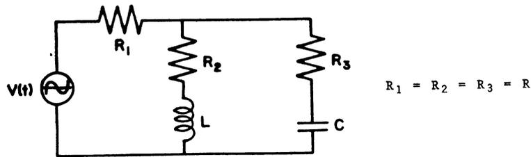
$$\frac{d^2 v_C}{dt^2} + \left[ \frac{3R}{2L} + \frac{1}{2RC} \right] \frac{dv_C}{dt} + \frac{1}{LC} v_C = \frac{1}{2LC} v(t) + \frac{1}{2RC} \dot{v}(t)$$
