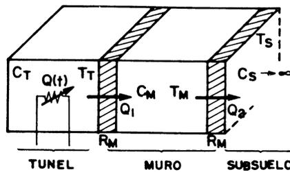
$$\frac{d^2 T_T}{dt^2} + \frac{C_M + 2C_T}{R_M C_M C_T} \frac{dT_T}{dt} + \frac{1}{R_M^2 C_M C_T} T_T = \frac{1}{C_T} \dot{Q}_0(t) + \frac{2}{C_M C_T R_M} Q_0(t) + \frac{1}{R_M^2 C_M C_T} T_S$$
