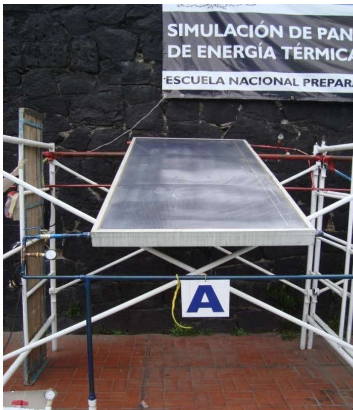
FIGURA 0.1 Colector solar “A”
