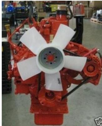
Figura 3.11 Perkins 402D-05 Tier 4 Diesel Engines [Perkins Engines Company]
