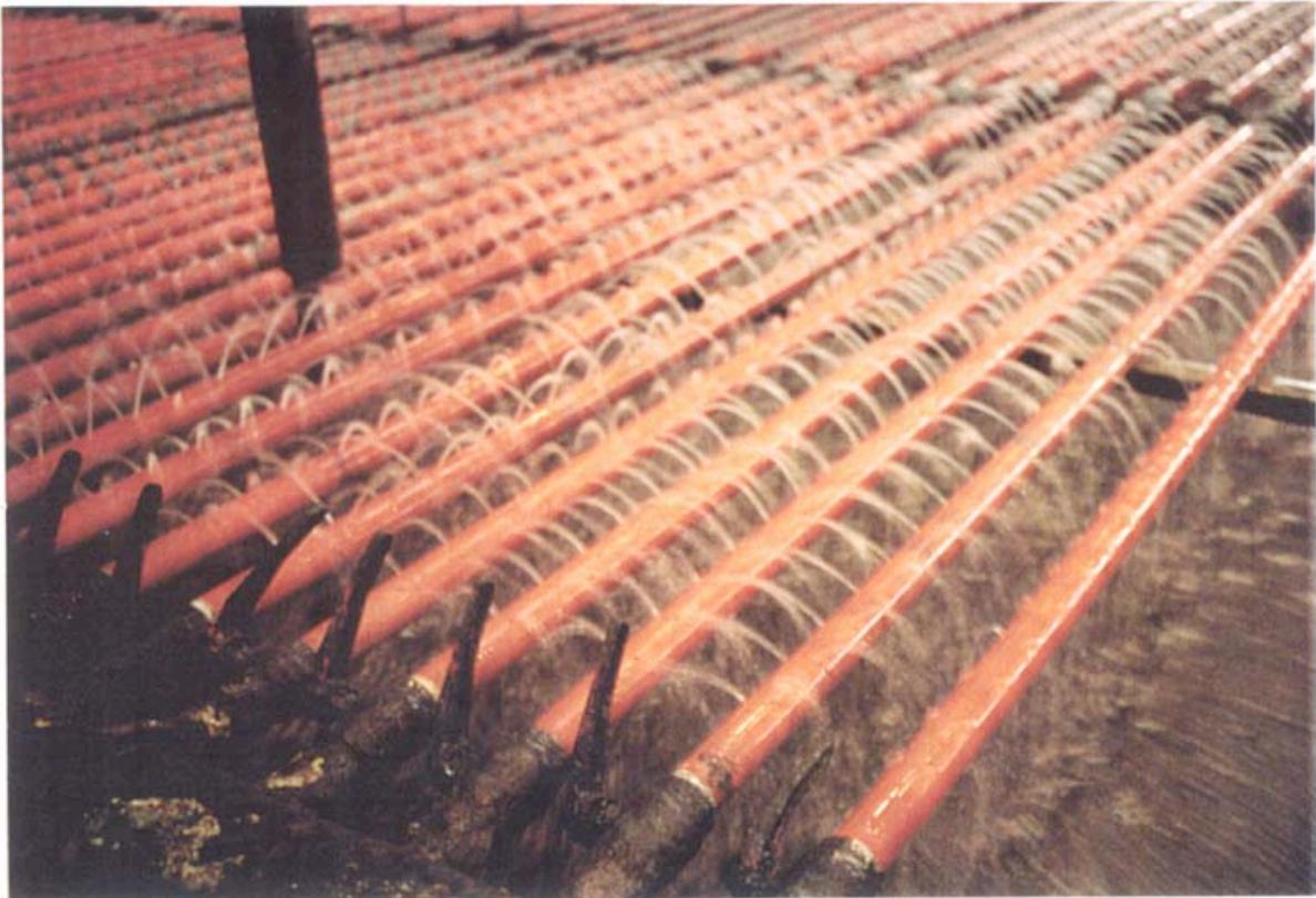
**Figura 3.24. Adición de agua de lavado (Tomada de Mineral producers improve plant performance using column flotation technology)**
