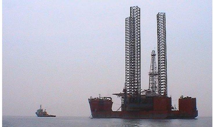
FIGURA 1.2-9 ARRASTRE O REMOLCADO SECO
