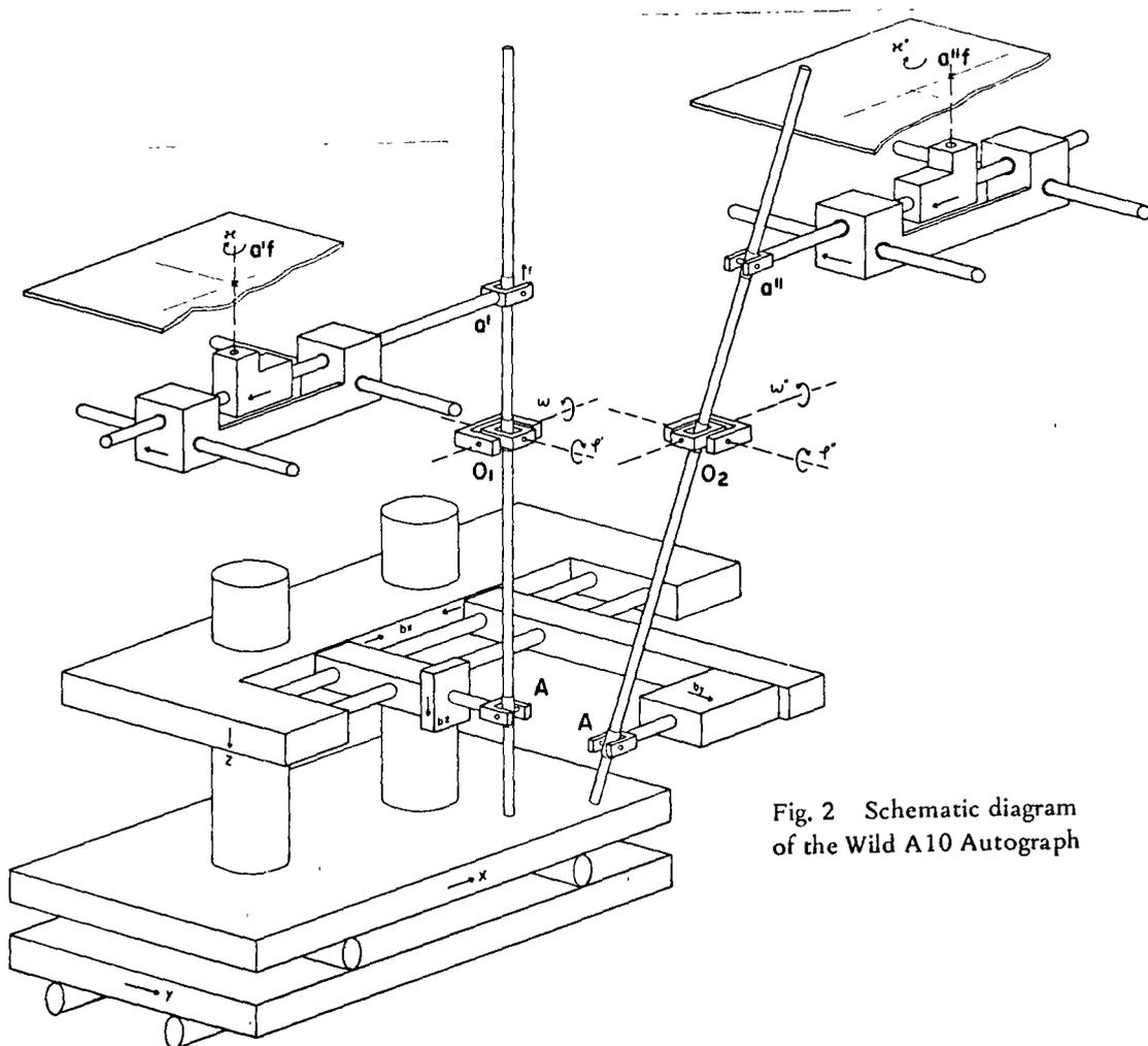
Fig. 2 Schematic diagram of the Wild A10 Autograph
