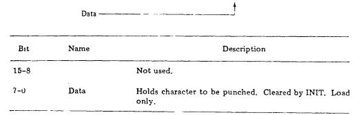
Any instruction that could modify TPB as a byte or word clears READY and initiates punching. Other references to either byte or word have no effect on the punch
