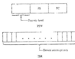
Fig. 6-16 Processor and interrupt status words
