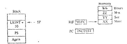
If the value in location MSEC is less than 59, it will be incremented by 1, . return made from the subroutine (e.g., the stack is popped) followed by a return from the interrupt routine (popping off the PC and PS from the stack). and the program will once again wait for an interrupt.
