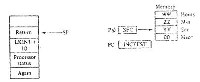
Again the value at the location pointed to by RC is checked to see if it is 59. If it is, it is zeroed, RO is advanced to point to the next most significant field.
