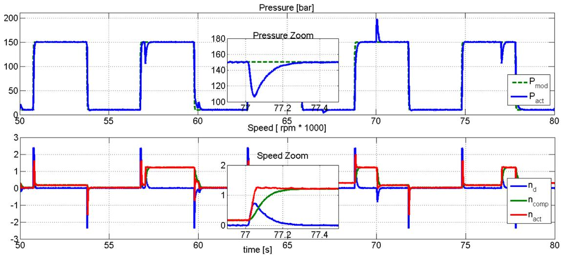
Figure 5.14: Response of the P-P cascade with the first order sliding mode compensator, the load valve opens and closes.
