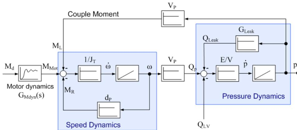
Figure 3.3: VsP Block diagram: the speed dynamics correspond to the pump coupled to the motor, the pressure dynamics correspond to the fixed volume. The main disturbance is the load flow  $Q_{LV}$  that is being taken out of the volume.
