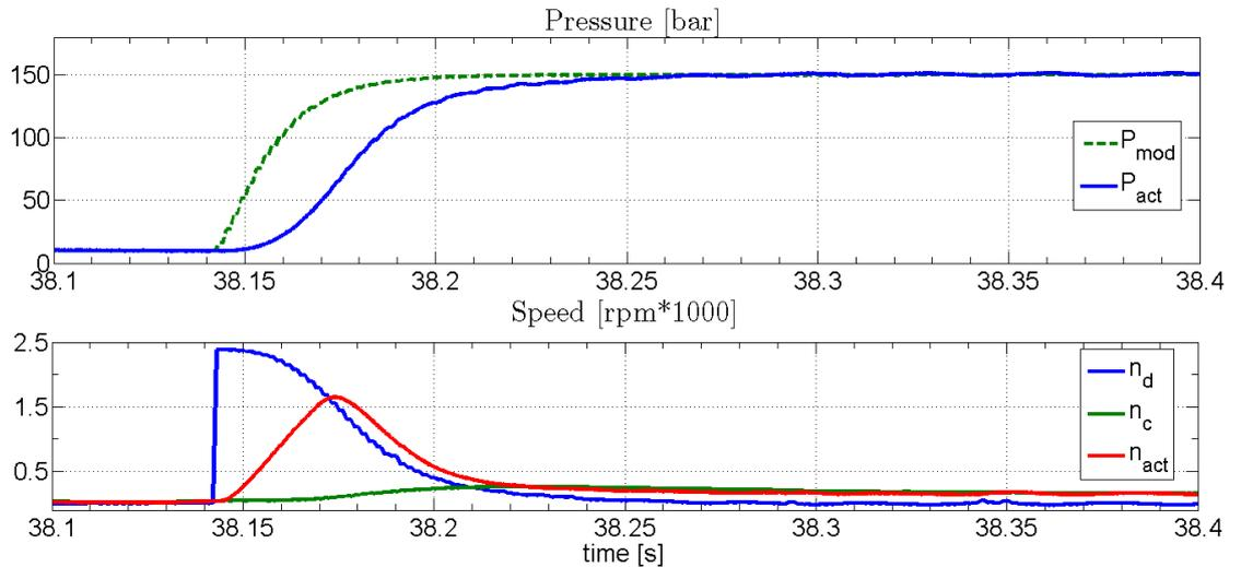
Figure 5.13: Zoom to the step response of the P-P cascade with the first order sliding mode compensator, the load valve is closed.
