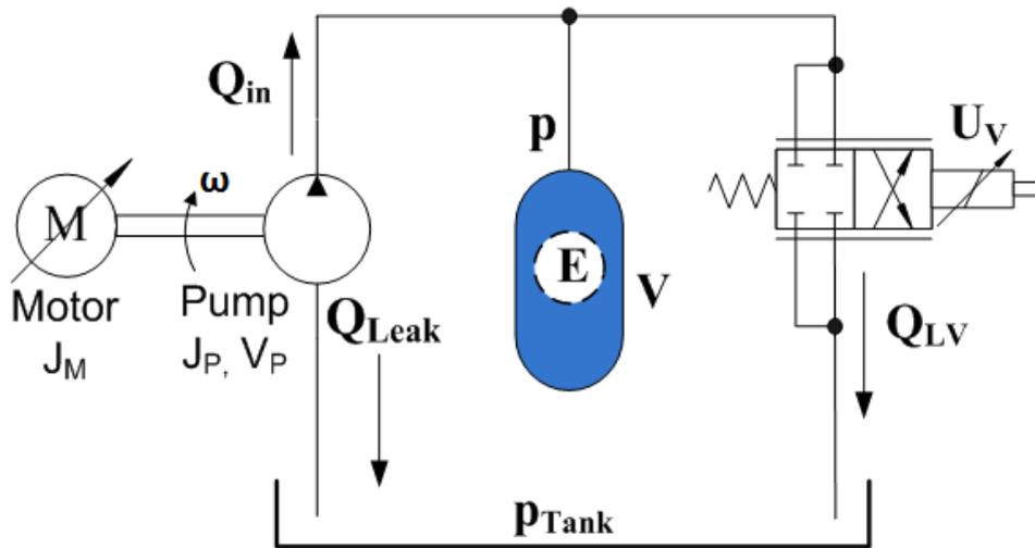
Figure 3.2: General hydraulic circuit for the VsP
