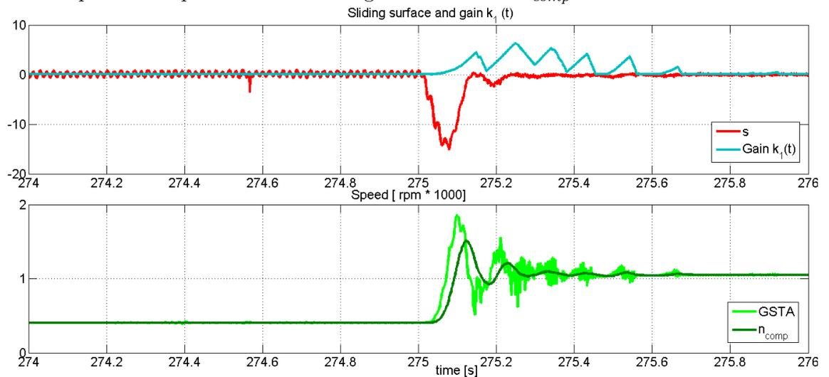
Figure 5.19: This figure is a zoom of the previous image. At the top are the gain  $k_1(t)$  of the generalized super twisting algorithm, and the sliding surface  $s$ . At the bottom the GSTA output and its filtered value  $n_{comp}$ .
