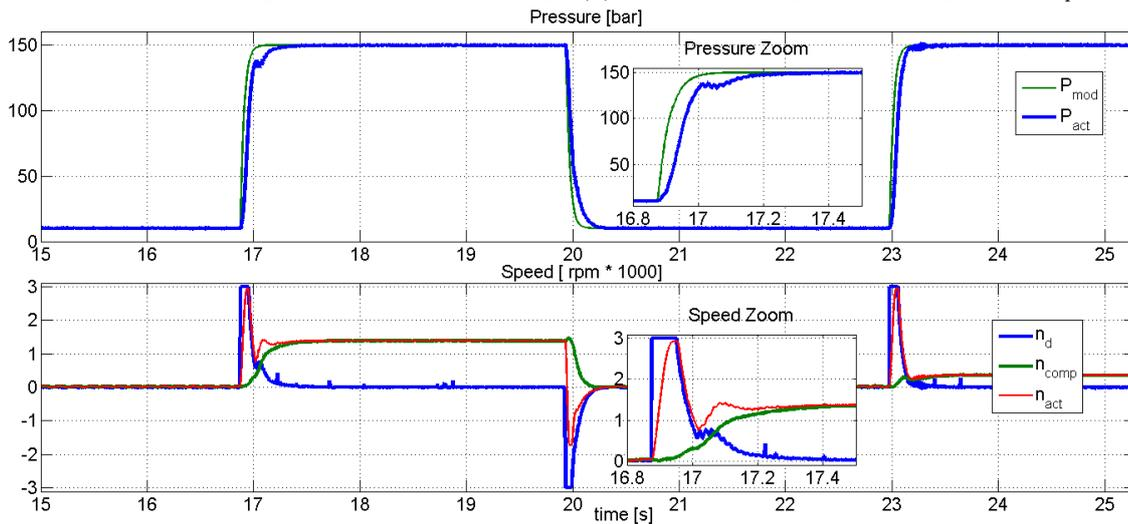
Figure 5.21: At the top the real pressure of the system, and the ideal pressure extracted from a closed loop model of the system. At the bottom the actual speed  $n_{act}$ , the demanded speed  $n_d$  from the linear feedback, and the compensation speed  $n_{comp}$  from the first order sliding mode observer. The zoom presents the moment when the pressure relief valve opens (at approximately  $t = 17$ ).
