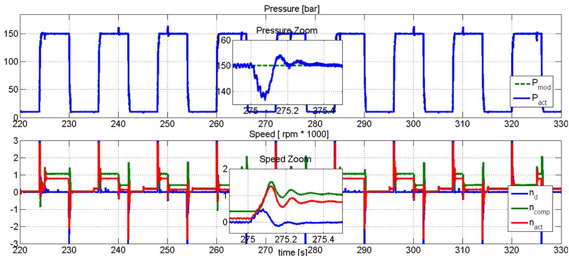
Figure 5.16: Response of the P-P cascade with the second order sliding mode compensator, the load valve opens and closes. The zoom window displays the disturbance (caused by the opening of the load valve) and the rejection by the compensation speed  $n_{comp}$ .
