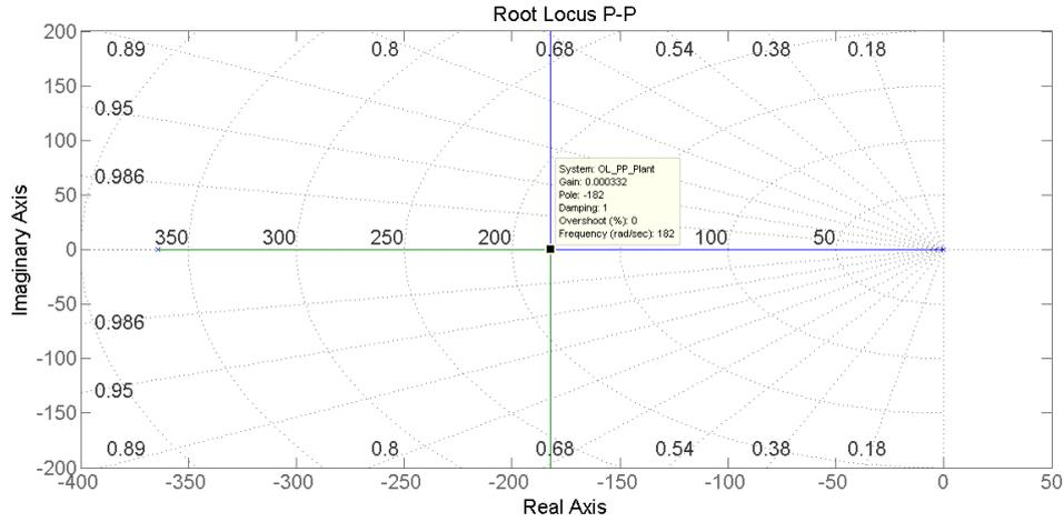
Figure 5.6: Root locus of the system using standard values of table 5.1, the inner loop features a fixed proportional control.
