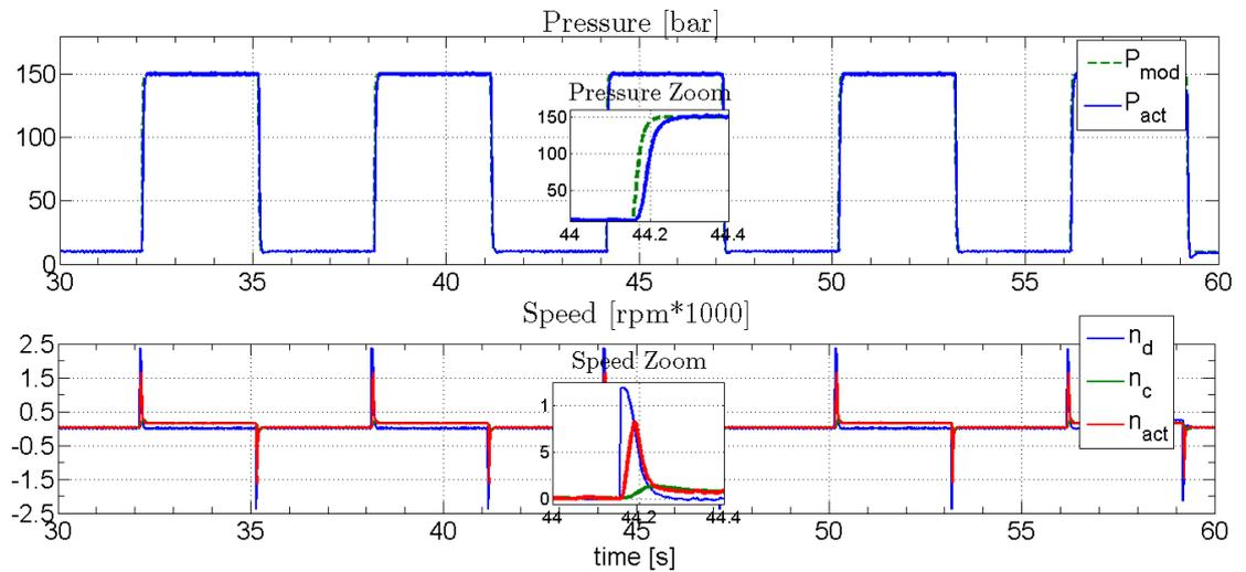
Figure 5.12: Response of the P-P cascade with the first order sliding mode compensator, the load valve is closed.
