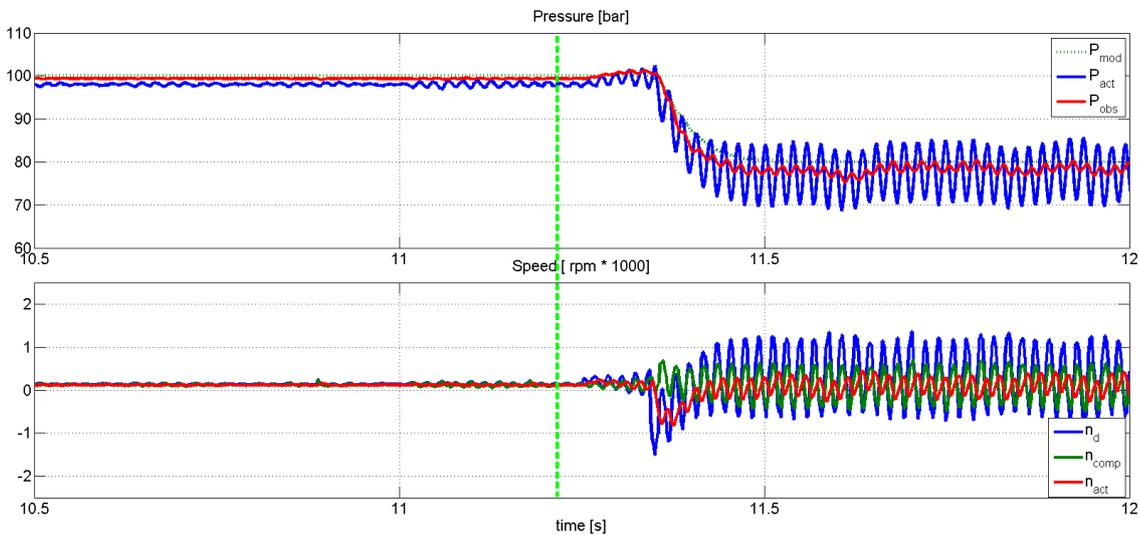
Figure 5.33: Zoom of the moment when the system becomes unstable, the green bar marks the moment when the compensation signal  $n_{comp}$  is given to the system.
