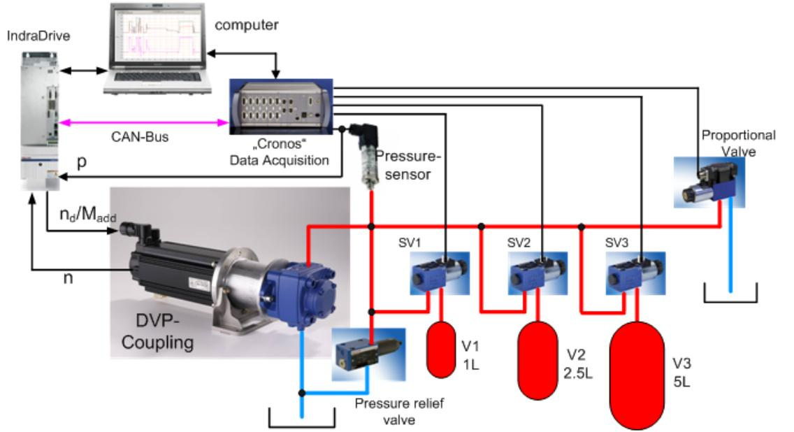
Figure 5.2: Test bench schematic
