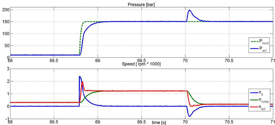
Figure 5.15: Zoom to the step response of the P-P cascade with the first order sliding mode compensator, the load valve is open before and after the step.
