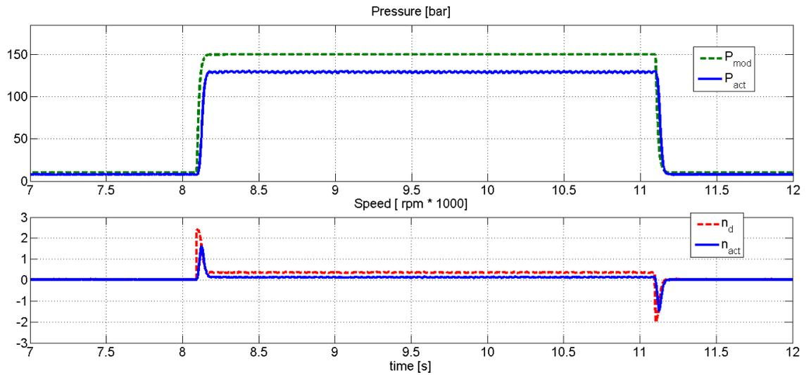
Figure 5.9: Response of the P-P cascade without sliding mode compensator, the load valve is closed.
