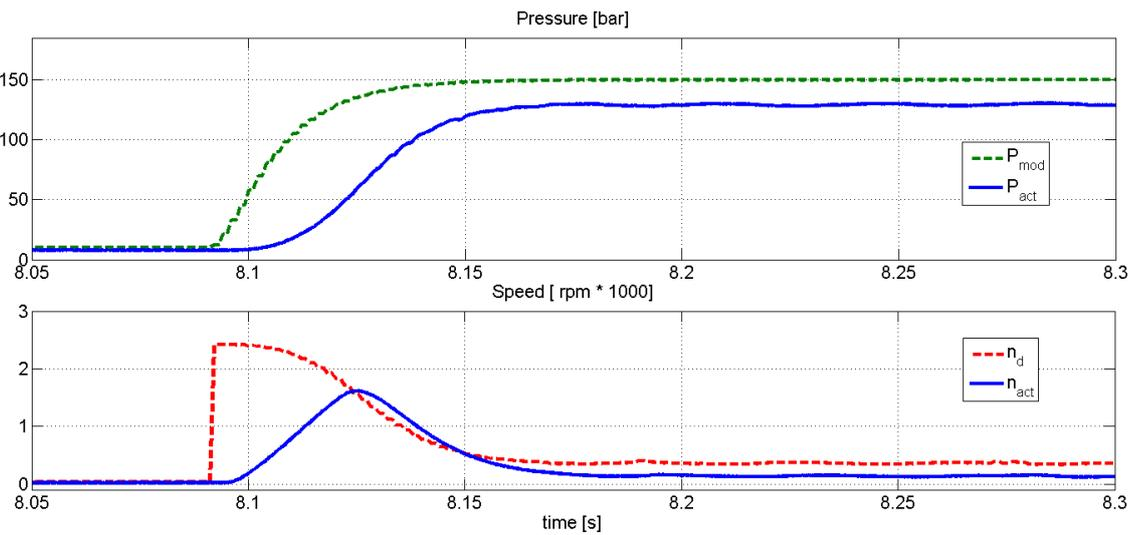
Figure 5.10: Zoom to the response of the P-P cascade without sliding mode compensator, the load valve is closed.
