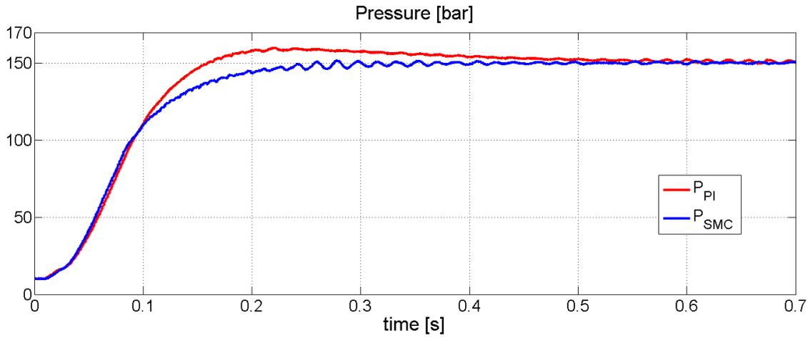
Figure 5.29: Comparison between the step response of the PI-P and the P-P plus sliding mode observer. The PI-P features an overshoot caused by the saturation of the motor's torque.
