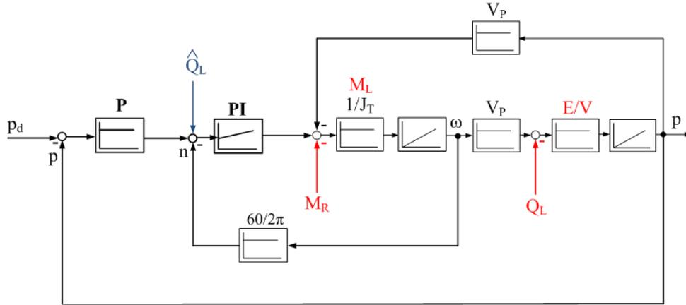
Figure 4.1: The cascade control with the feed forward of the estimated load flow  $\hat{Q}_L$ .
