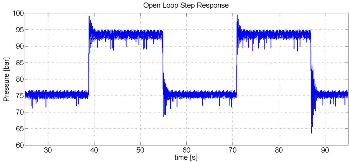
Figure 5.3: Open loop step response showing the output pressure of the system when the input  $M_{in}$  is applied, The desired pressure  $P_d$  is a rectangular signal from 80 [bar] to 100 [bar]
