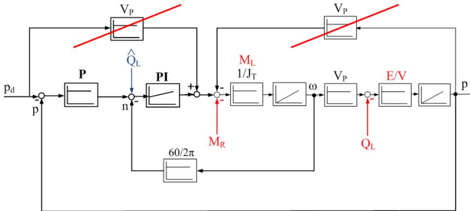
Figure 4.2: The control scheme with the feedforward of the couple moment, the couple moment cancels the moment due to pressure.
