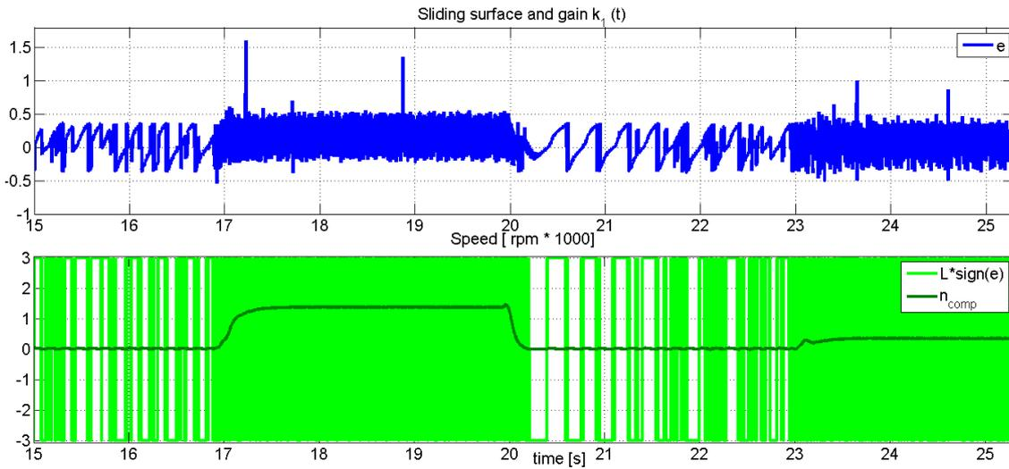
Figure 5.20: At the top the sliding surface  $e$ , at the bottom the discontinuous signal from the first order sliding mode observer  $L \cdot \text{sign}(e)$ , and the compensation signal  $n_{comp}$ .
