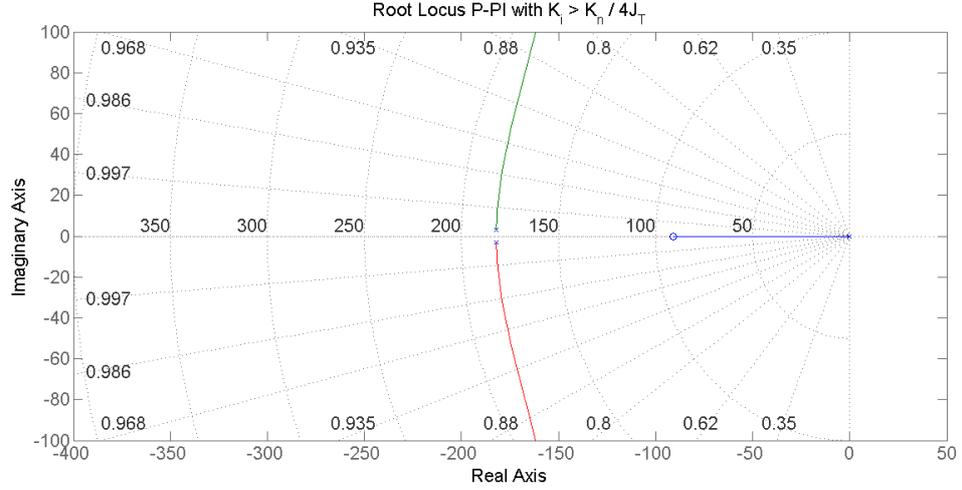
Figure 5.8: Root locus of the system using standard values of table 5.1, the inner loop features a proportional plus integral control, the integral gain  $K_i$  is equal to 100.
