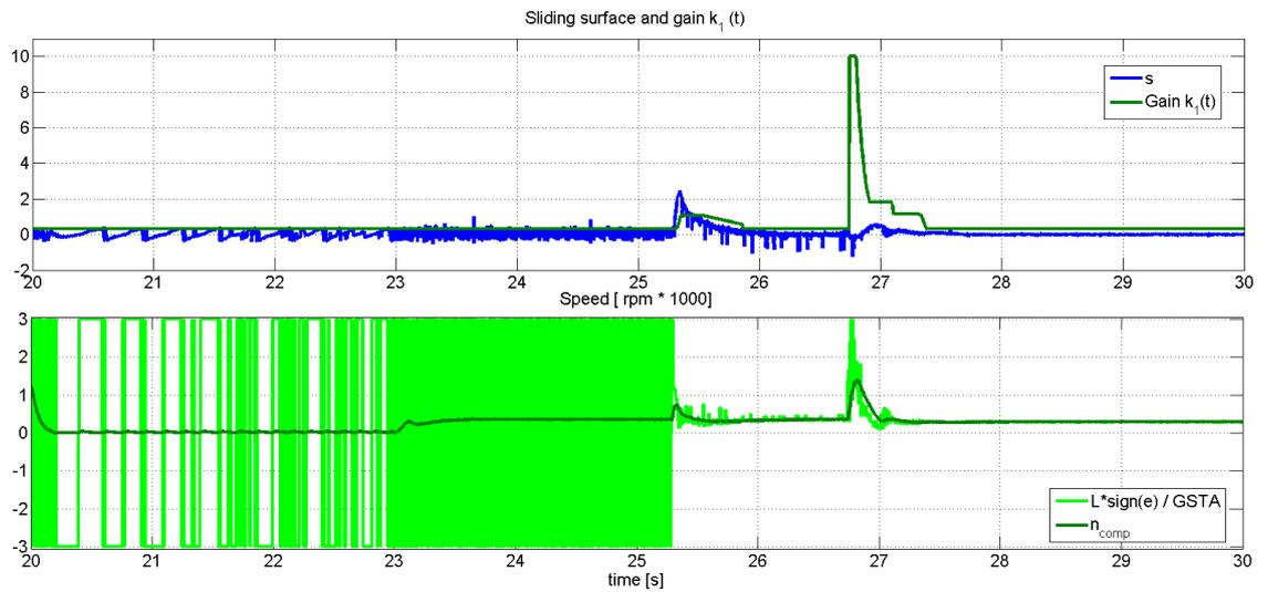
Figure 5.22: Here the switch is being made between first order sliding mode and second order sliding mode while the machine is operating (between second 25 and 26). At the top the sliding surface  $e$ , at the bottom the discontinuous signal from the first order sliding mode observer  $L \cdot \text{sign}(e)$ , and the compensation signal  $n_{comp}$ .
