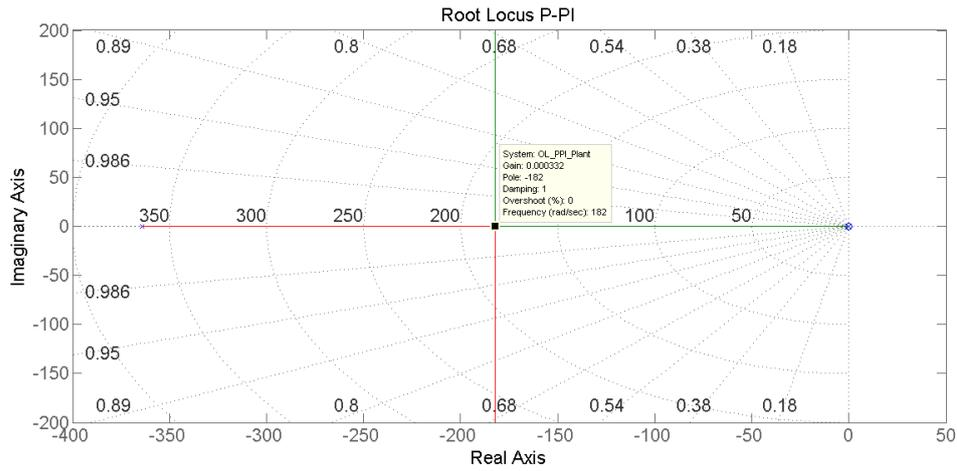
Figure 5.7: Root locus of the system using standard values of table 5.1, the inner loop features a proportional plus integral control, the integral gain  $K_i$  is equal to 0.0625.
