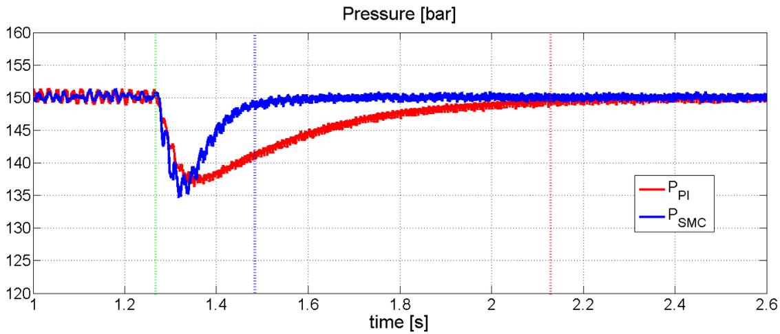
Figure 5.30: Response of the PI-P when the proportional valve opens, the P-P plus sliding mode observer is approximately four times faster.
