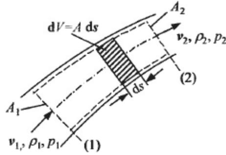
Figure 2.2: Flow in a control tube
