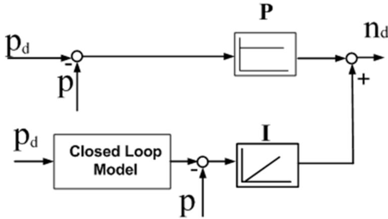
Figure 5.28: Scheme of the modified PI-P.
