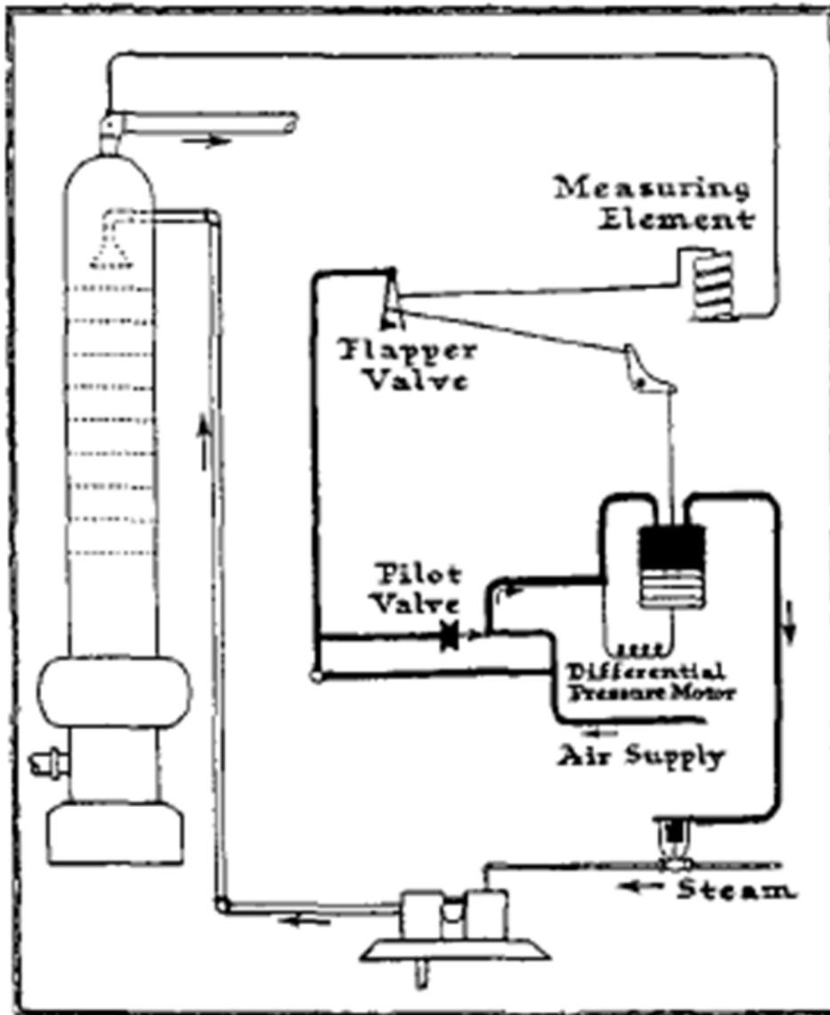
Figure 1.1: Control PI explained in 1934, taken from [1]
