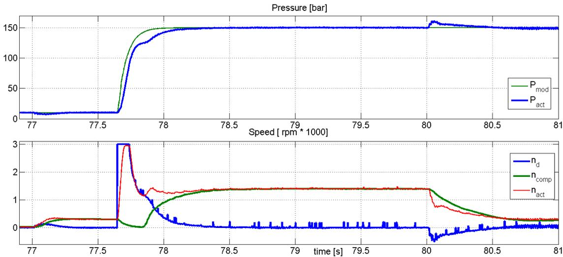
Figure 5.26: The rising step. At the top the real pressure of the system  $P_{act}$ , and the ideal pressure extracted from a closed loop model of the system  $P_{mod}$ . At the bottom the actual speed  $n_{act}$ , the demanded speed  $n_d$  from the linear feedback, and the compensation speed  $n_{comp}$  from the second order sliding mode observer.
