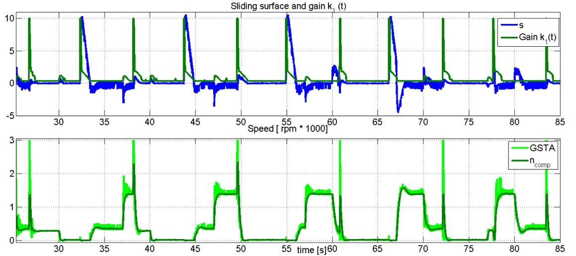
Figure 5.24: At the top the sliding surface  $s$ , at the bottom the output of the generalized super twisting algorithm from the second order sliding mode observer, and the compensation signal  $n_{comp}$ .
