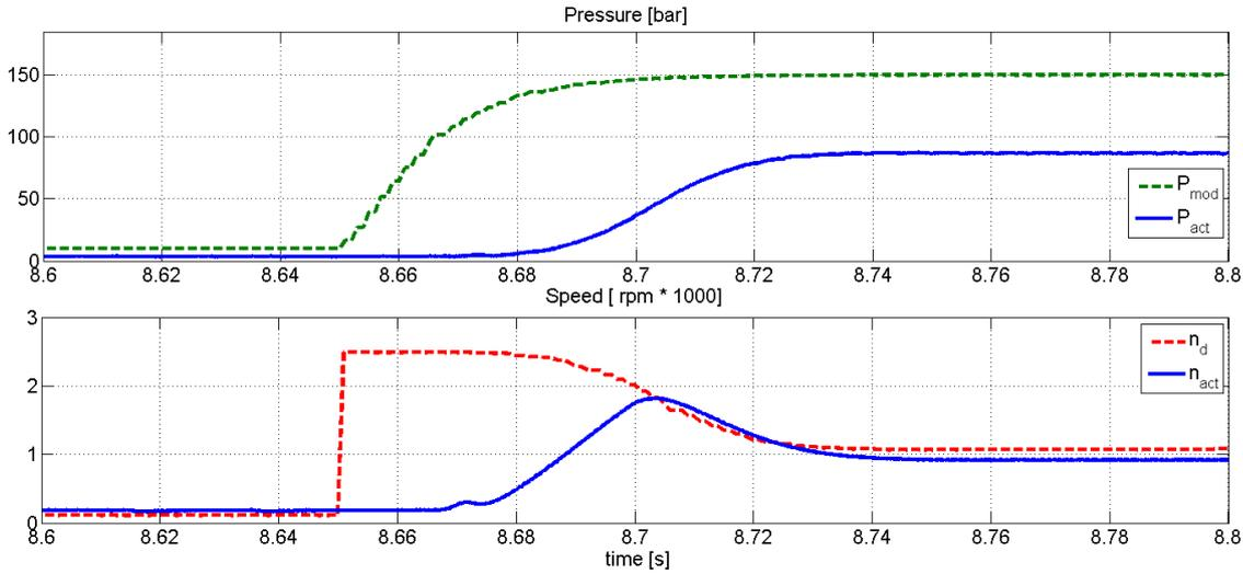
Figure 5.11: Response of the P-P cascade without sliding mode compensator, the load valve is open.
