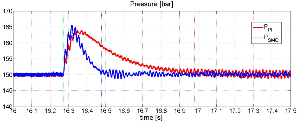
Figure 5.31: Response of the PI-P when the proportional valve closes, the P-P plus sliding mode observer is approximately four times faster.
