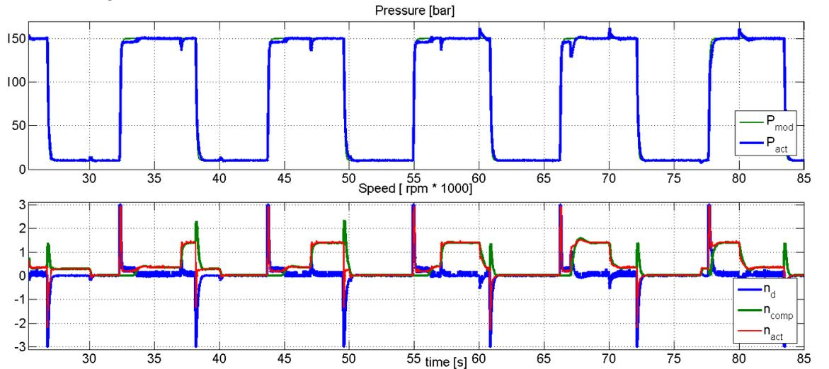
Figure 5.25: At the top the real pressure of the system  $P_{act}$ , and the ideal pressure extracted from a closed loop model of the system  $P_{mod}$ . At the bottom the actual speed  $n_{act}$ , the demanded speed  $n_d$  from the linear feedback, and the compensation speed  $n_{comp}$  from the second order sliding mode observer.
