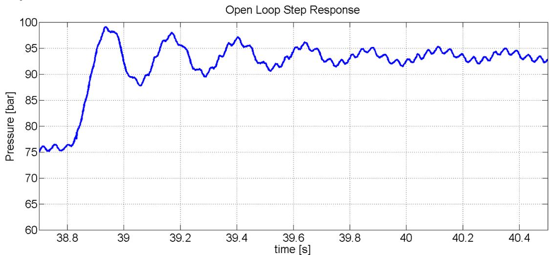
Figure 5.4: Zoom of the open loop step response showing the output pressure of the system
