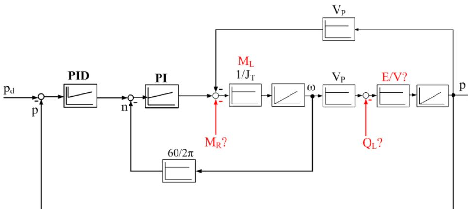
Figure 3.4: The standard solution for this kind of System is the cascade control, in this case the inner loop features a PI that controls the motors velocity, the outer loop features a PID that controls the system pressure.
