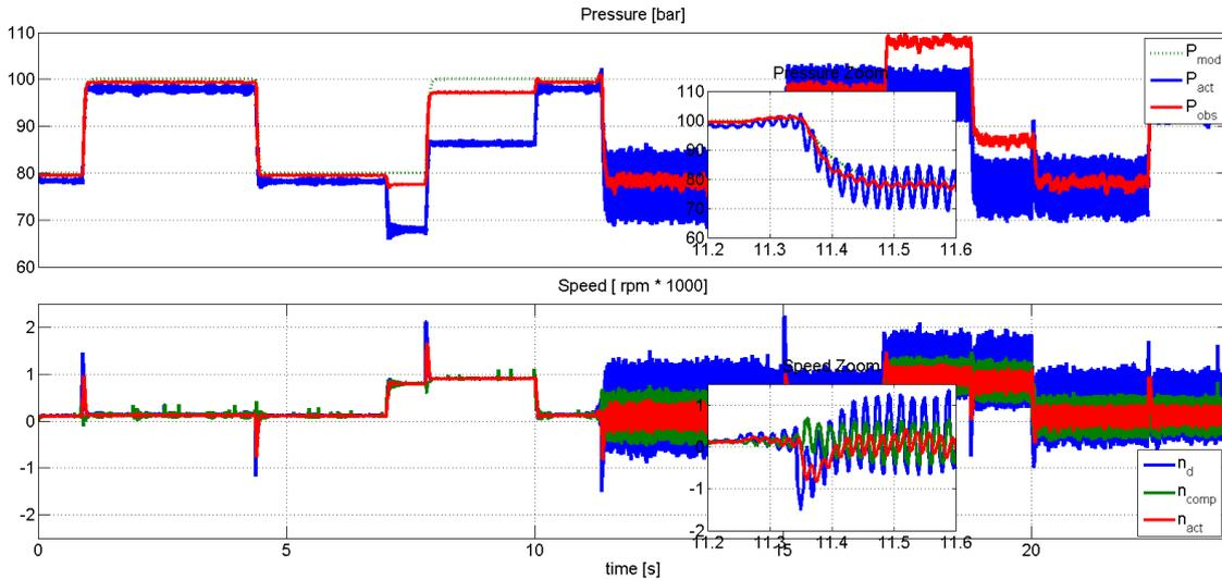
Figure 5.32: Before 11.2 [s] the linear observer is working but the compensation signal  $n_{comp}$  (from the linear observer) is not feeded to the system. Adter 11.2 [s] the compensation signal  $n_{comp}$  is given to the system, the system become marginally stable (In practical applications this behavior is considered unstable).
