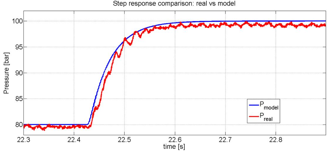
Figure 5.5: Comparison between the real plant step response and the model. The displayed scale correspond to the model, the real plant response has been scaled in magnitude.
