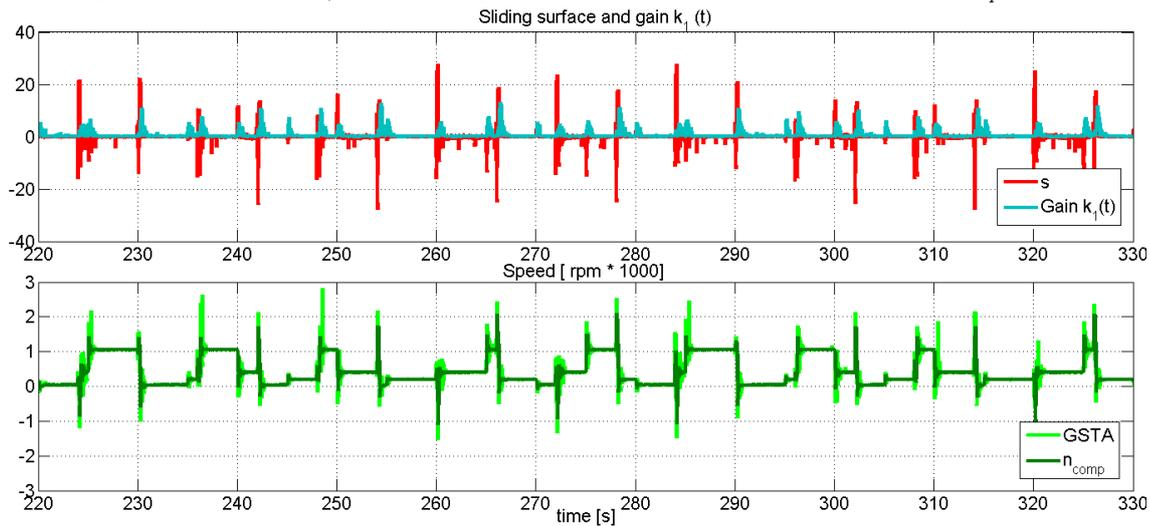
Figure 5.17: At the top are the gain  $k_1(t)$  of the generalized super twisting algorithm, and the sliding surface  $s$ . At the bottom the GSTA output and its filtered value  $n_{comp}$ . The period of time for these graphics is the same as the previous image.
