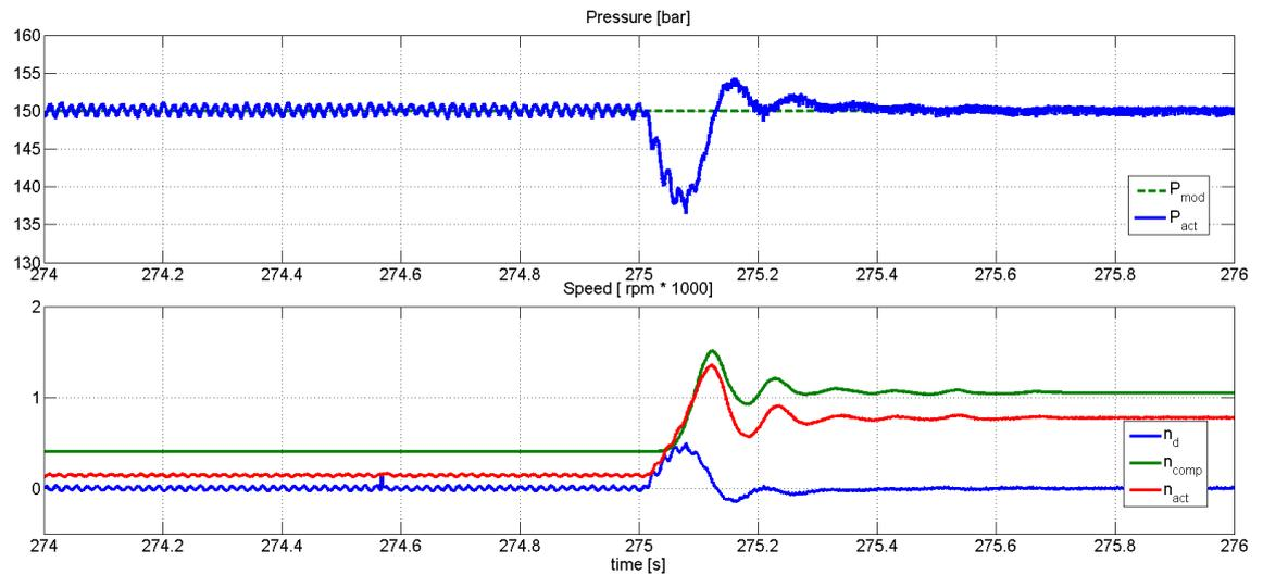
Figure 5.18: This figure is a zoom of the previous figure 5.16. At the top are the actual pressure  $P_{act}$  of the system, and the ideal pressure from the disturbance free model  $P_{mod}$ . At the bottom the actual speed  $n_d$ , the demanded speed from the linear scheme  $n_d$ , and the compensation speed from the sliding mode observer  $n_{comp}$ .
