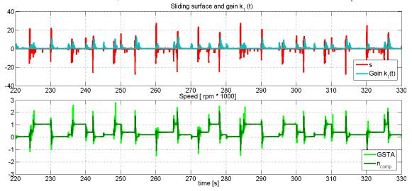
Figure 5.17: At the top are the gain  $k_1(t)$  of the generalized super twisting algorithm, and the sliding surface s. At the bottom the GSTA output and its filtered value  $n_{comp}$ . The period of time for these graphics is the same as the previous image.
