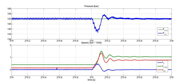
Figure 5.18: This figures is a zoom of the previous figure 5.16. At the top are the actual pressure  $P_{act}$  of the system, and the ideal pressure from the disturbance free model  $P_{mod}$ . At the bottom the actual speed  $n_d$ , the demanded speed from the linear sheem  $n_d$ , and the compensation speed from the sliding mode observer  $n_{comp}$ .
