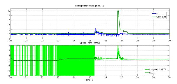
Figure 5.22: Here the switch is being made between first order sliding mode and second order sliding mode while the machine is operating (between second 25 and 26). At the top the sliding surface e, at the bottom the discontinuous signal from the first order sliding mode observer  $L \cdot sign(e)$ , and the compensation signal  $n_{comp}$ .
