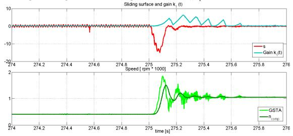
Figure 5.19: This figures is a zoom of the previous image. At the top are the gain  $k_1(t)$  of the generalized super twisting algorithm, and the sliding surface s. At the bottom the GSTA output and its filtered value  $n_{comp}$ .
