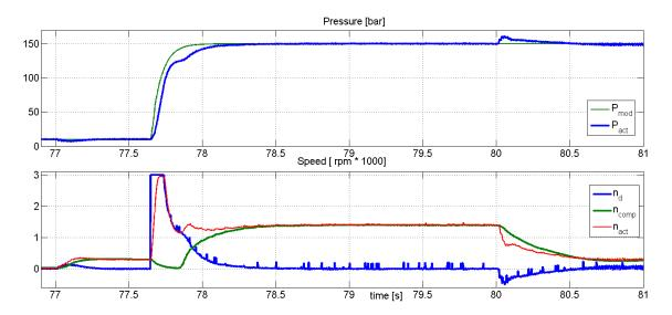
Figure 5.26: The rising step. At the top the real pressure of the system  $P_{act}$ , and the ideal pressure extracted from a closed loop model of the system  $P_{mod}$ . At the bottom the actual speed  $n_{act}$ , the demanded speed  $n_d$  from the linear feedback, and the compensation speed  $n_{comp}$  from the second order sliding mode observer.
