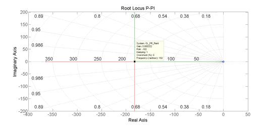
Figure 5.7: Root locus of the system using standard values of table 5.1, the inner loop features a proportional plus integral control, the integral gain  $K_i$  is equal to 0.0625.
