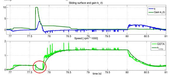
Figure 5.27: The rising step (same as the previous plot). At the top the sliding surface e (displayed as s), and the gain  $k_1(t)$ . At the bottom the output v of the GSTA, and its filtered value  $n_{comp}$ ; notice the red circle, it indicates the moment when the GSTA goes off due to safety reasons (the speed is hitting the maximal value of 3000 [rpm]), after the speed returns to normal operation values, the algorithm starts working again without any overshoot or aggressive oscillations.
