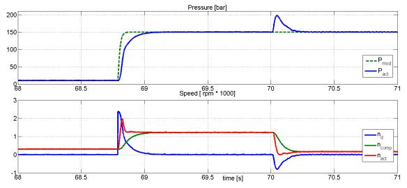
Figure 5.15: Zoom to the step response of the P-P cascade with the first order sliding mode compensator, the load valve is open before and after the step.
