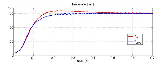
Figure 5.29: Comparison between the step response of the PI-P and the P-P plus sliding mode observer. The PI-P features an overshoot caused by the saturation of the motor's torque.
