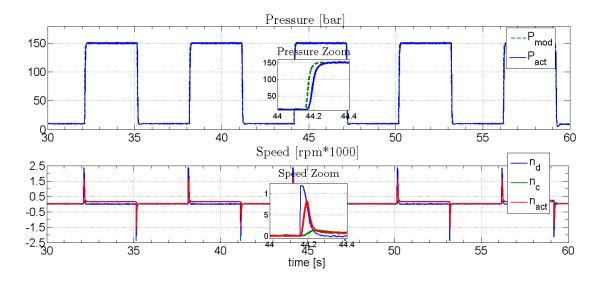
Figure 5.12: Response of the P-P cascade with the first order sliding mode compensator, the load valve is closed.
