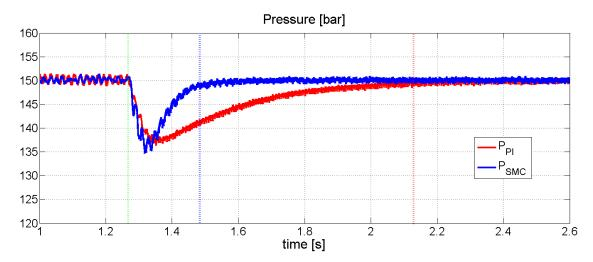
Figure 5.30: Response of the PI-P when the proportional valve opens, the P-P plus sliding mode observer is approximately four times faster.
