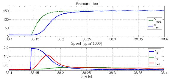
Figure 5.13: Zoom to the step response of the P-P cascade with the first order sliding mode compensator, the load valve is closed.
