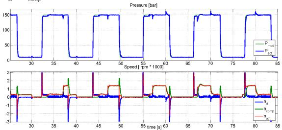
Figure 5.25: At the top the real pressure of the system  $P_{act}$ , and the ideal pressure extracted from a closed loop model of the system  $P_{mod}$ . At the bottom the actual speed  $n_{act}$ , the demanded speed  $n_d$  from the linear feedback, and the compensation speed  $n_{comp}$  from the second order sliding mode observer.
