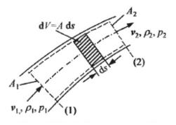
Figure 2.2: Flow in a control tube
