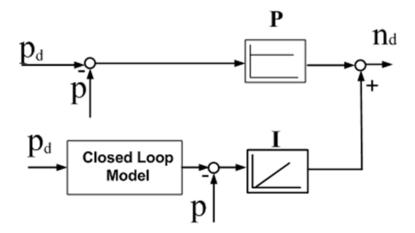
Figure 5.28: Scheme of the modified PI-P.
