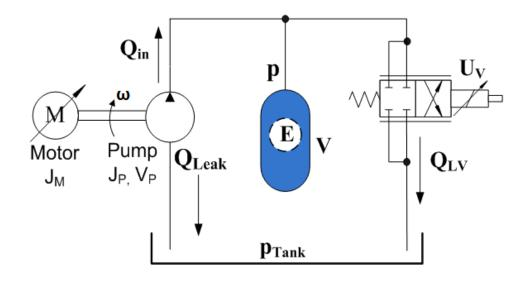
Figure 3.2: General hydraulic circuit for the VsP
