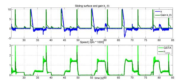
Figure 5.24: At the top the sliding surface s, at the bottom the output of the generalized super twisting algorithm from the second order sliding mode observer, and the compensation signal  $n_{comp}$ .
