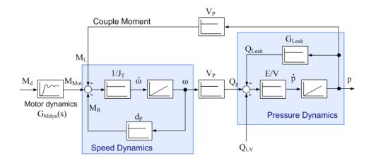
Figure 3.3: VsP Block diagram: the speed dynamics correspond to the pump coupled to the motor, the pressure dynamics correspond to the fixed volume. The main disturbance is the load flow  $Q_{LV}$  that is being taken out of the volume.
