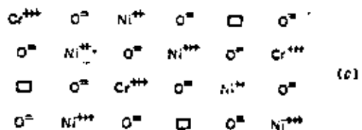
Fig. 11-8. Idealized lattice structure of nickel oxide, a p-type semiconductor. (a) Pure NiO; (b) effect of Li + additions; (c) effect of Cr 3+ additions.
