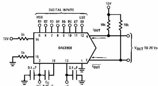
FIGURE 1.  $\pm 20$  V<sub>p-p</sub> Output Digital-to-Analog Converter (Note 5)
