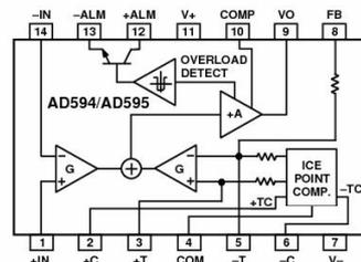
are available at the package pins so that the circuit can be recalibrated for the thermocouple types by the addition of two or three resistors. These terminals also allow more precise calibration for both thermocouple and thermometer applications.
