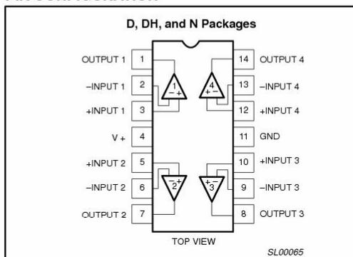
Figure 1. Pin configuration.
