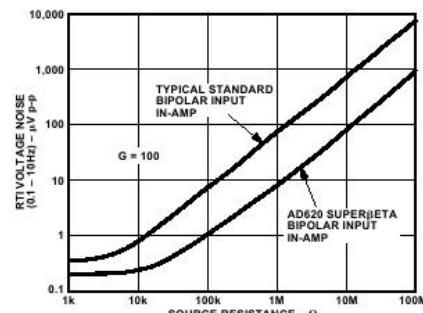
Figure 2. Total Voltage Noise vs. Source Resistance
