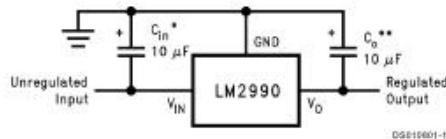
\*Required if the regulator is located further than 6 inches from the power supply filter capacitors. A 1 μF solid tantalum or a 10 μF aluminum electrolytic capacitor is recommended.
