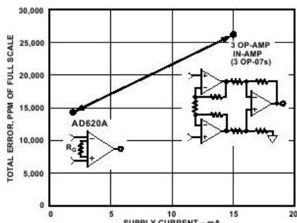
Figure 1. Three Op Amp IA Designs vs. AD620
