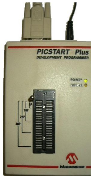
Figura 5.7 Programador PICSTART PLUS.
