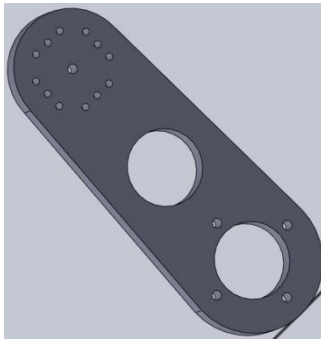
Figure 11. Primary link of the Spatial Parallel Manipulator
