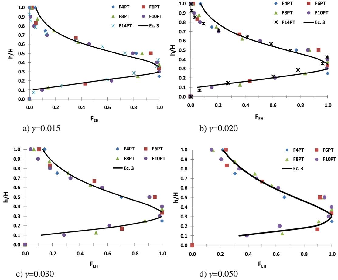
Fig. 12 Comparison of  $F_{EH}$  using Eq. (3) with the result of the numerical analysis for all the models and several values of  $\gamma$ .
