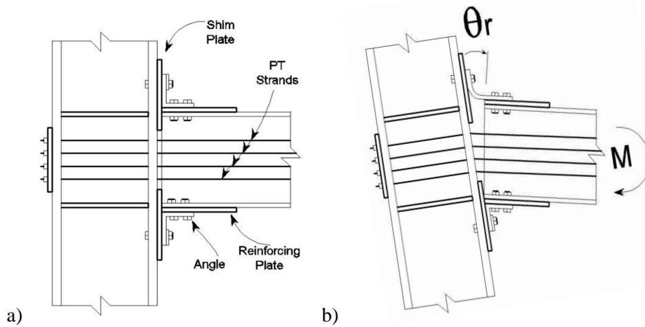
Fig. 4 PT connection a) Original configuration, b) Deformed configuration
