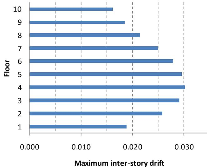
Fig. 6 Inter-story drift in F10PT under record 1 scaled to  $Sa(T_1)=1.3g$
