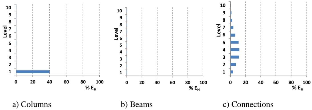
Fig. 10  $E_H$  dissipated in each level of F10PT by columns, beams and connections for a target median  $\gamma = 0.030$
