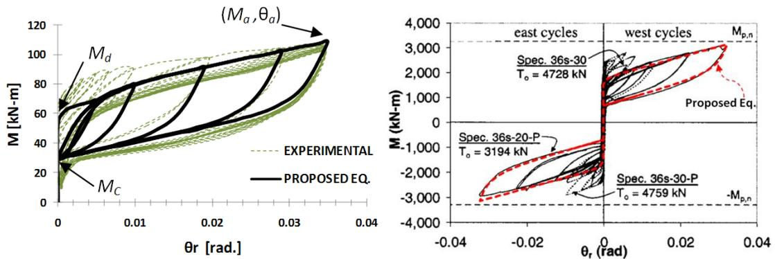
a) Proposed equations and experimental results      b) Proposed equations and Garlock results
