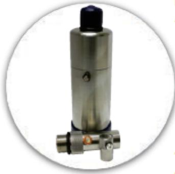
High Frequency Transducers offer frequency ranges from 30MHz to 150MHz. Applications include acoustic microscopy, flaw detection, and characterization of solder bumps in flip-chips in the microelectronics industry, high resolution thickness of meals down to 0.001" (0.0254mm), and high resolution surface wave imaging.
