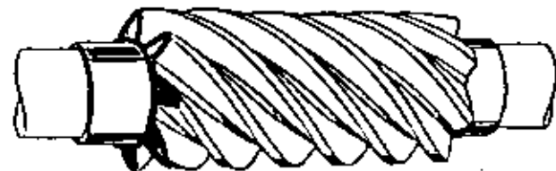
Fig. 43 . . . Multiple-Thread Worm. Eight teeth or threads are machined on this worm.
