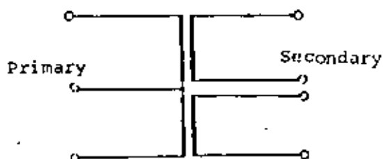
Fig. 3-6 V Connection Transformer
