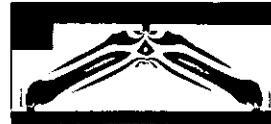
Model M-247: Knee frame . . . for teaching stress distribution in typical structural shapes.
