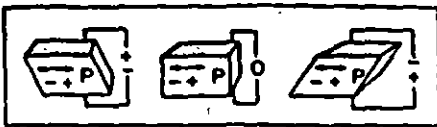
Figure 3. It is possible to produce various stresses and strains in the material by means of different combinations of the orientation of the crystal and the direction of the applied field. In this example, a field applied parallel to the piezoelectric axis produces elongation in the direction of the axis.
