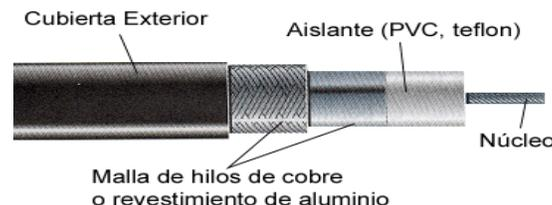
Figura 17 Componentes del Cable Coaxial
