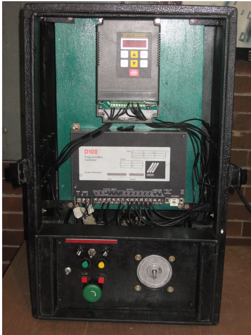
Figura 142 Sistema PLC – Drive – Motor.
