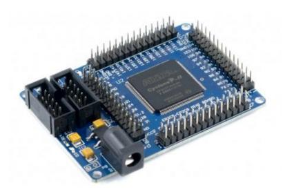
Figura 1.2 FPGA Cyclone II de ALTERA
