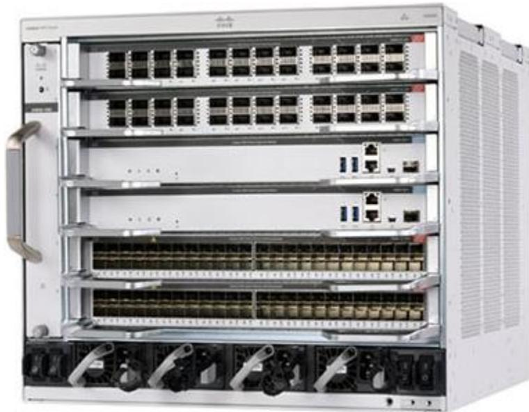
Figura 4.7: Switch Modelo Catalyst 9600 [23].
