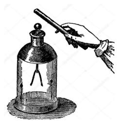
Figura 1.1 Electroscopio [3]
